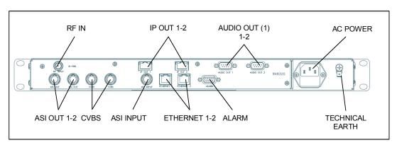
Figure 1 Rear Panel Connectors
